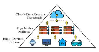
Fig. 1. Typical edge computing architecture.
